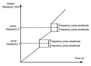
Fig. 6-18 Diagram for valid hopping frequency during acceleration/deceleration
