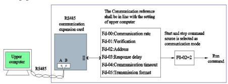
Fig. 4-7 The example of start and stop control mode of the communication
