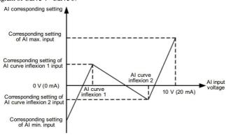
Fig. 6-33 Diagram of Curve 4 and Curve 5
