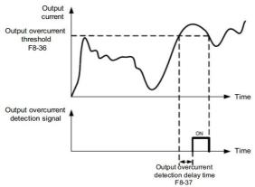
Fig. 6-22 Output current over limit test diagram
