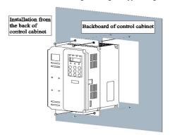
Fig. 3-5 The diagram of embedded installation of plastic structure
