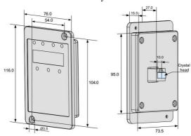
Fig. 8-3 The overall dimensions of introduced keyboard
