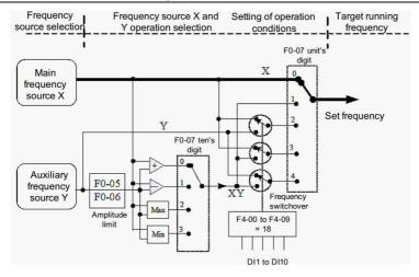
When make frequency source as main and auxiliary operation, can set offset frequency by F0-21. Superimpose offset frequency base on the result of main and auxiliary operation to cope with various demand.
