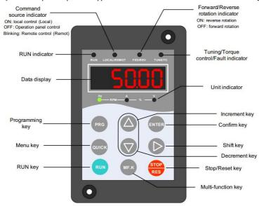
Fig. 4-1 Operation panel diagram
