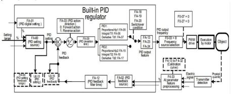
Fig. 4-22 The closed-loop control of frequency of process control
