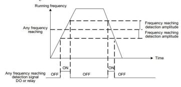
Fig. 6-20 Arbitrarily arriving frequency test diagram
