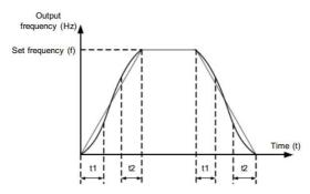
Fig. 6-11 Diagram for S-curve acceleration/deceleration A
