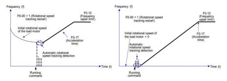
Fig. 4-9 Speed tracking restart mode
