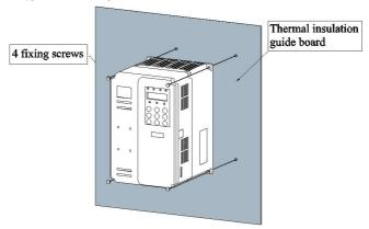
Fig. 3-3 Wall-mounted type installation diagram of plastic structure
