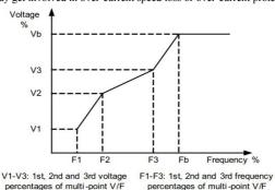
Fig. 6-4 Multi-point V/F curve setting diagram
