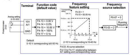
Fig. 4-19 Function code setting of AI1 voltage input frequency reference
