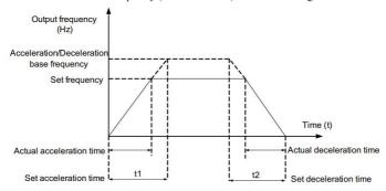
Fig. 6-1 Acceleration/deceleration time diagram
