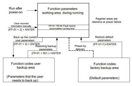
Fig. 4-32 Parameter backup and recovery setting
