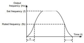
Fig. 6-12 Diagram for S-curve Acceleration/Deceleration B
