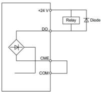
Fig. 3-27 The wiring diagram of digital output terminal
