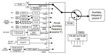
Fig. 4-17 Selection of given auxiliary frequency source
