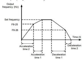
Fig. 6-19 Acceleration/deceleration time switching diagram
