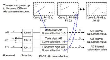
Fig. 4-30 The actual reference corresponding to AI signal
