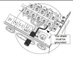
Fig. 7-1 The diagram for shield cable grounding
