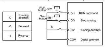
Fig. 6-9 Three-line control mode 2
