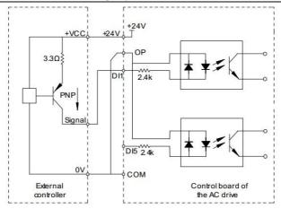
Fig. 3-26 Active wiring mode
