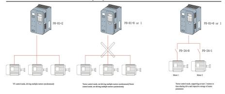
Fig. 4-29 Multi-motor switching
