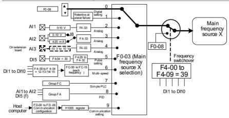
Fig. 4-16 Selection of given main frequency source
