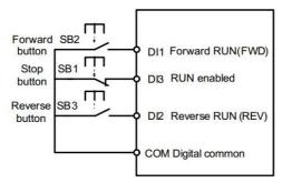
Fig. 6-8 Three-line control mode 1
