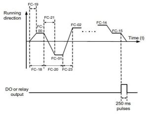
Fig. 6-31 Simple PLC Diagram
