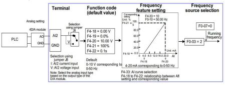
Fig. 4-20 Function code setting of AI2 current type input frequency reference
