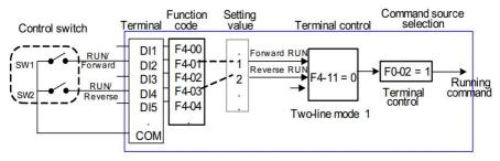
Fig. 4-5 The examples of start and stop control mode of the terminal
