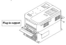
Fig. 3-4 Plug-in support diagram of plastic structure installation
