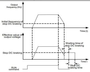
Fig. 6-13 Stop DC braking diagram
