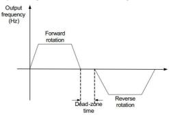
Fig. 6-15 Forward/Reverse Running Dead Time Diagram
