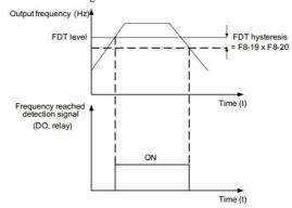
Fig. 6-16 FDT level diagram
