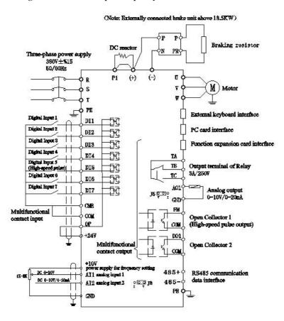
Fig. 3-21Control loop wiring mode of frequency converter
