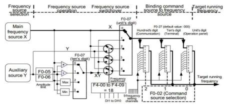
Fig. 4-18 Selection of the given mixed source of main/auxiliary frequency
