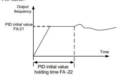
Fig 6-28: The diagram of PID starter function
