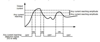
Fig. 6-23 Arbitrarily arriving frequency test diagram
