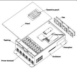
Fig. 2-3 The outline drawing of sheet metal structure of 580 series frequency converter
