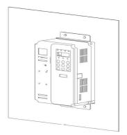
Fig. 3-6 Embedded installation effect chart of plastic structure
