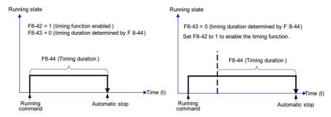
Fig. 4-12 Timing stop function
