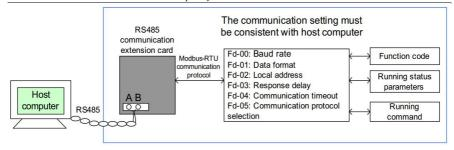
Fig. 4-31 The usage of serial communication of frequency converter
