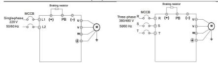
Fig. 3-16 Single 0.75-2.2kW wiring standard
