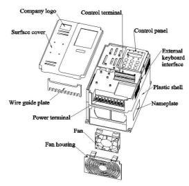
Fig. 2-2 The outline drawing of plastic structure of 580 series frequency converter
