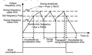
Fig. 6-29 Swing frequency diagram
