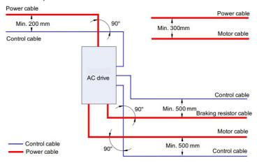
Fig. 7-2 Cables distribution
