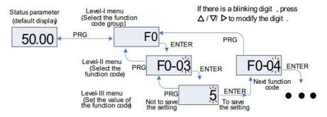
Fig. 4-2 The operation flow chart of three-level menus
