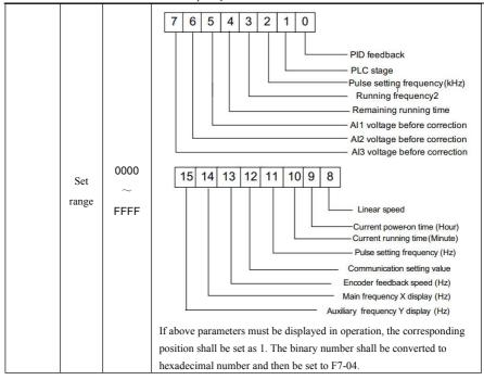
Displayed parameters in operation shall be used to set the parameters that can be checked when the frequency converter is in operation.
