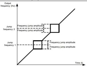
Fig. 6-14 Hopping frequency diagram
