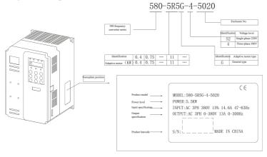
Fig. 2-1 Naming and nameplate identification
