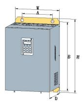
Fig. 8-2 metal plate structure appearance dimension and installation dimension of 580 series
