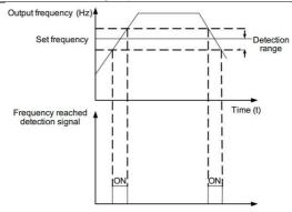
Fig. 6-17 Diagram for detected amplitude of frequency arrival
