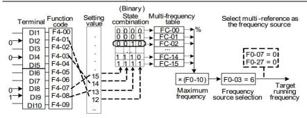
Fig. 4-24 Multi-speed mode setting
