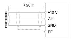
Fig. 3-22 The wiring diagram of analog input terminal
