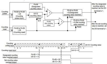
Fig. 4-28 Function code setting of count mode
