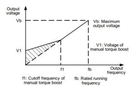
Fig. 6-3 Manual torque boost diagram
