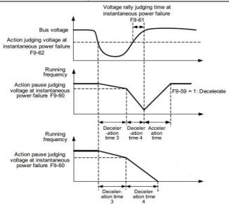
Fig. 6-25 The diagram of instantaneous power failure action
