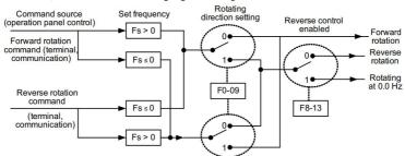
Fig. 4-25 Setting the running direction of motor
