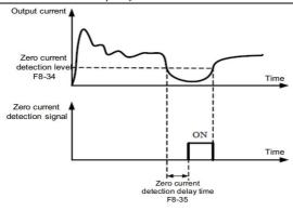
Fig. 6-21 Zero current test diagram
